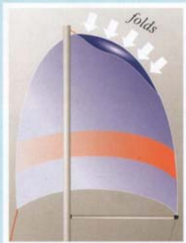
Pole too low
