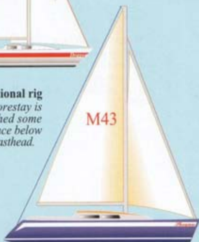
Masthead rig Backstay and forestay are both attached at the masthead.
