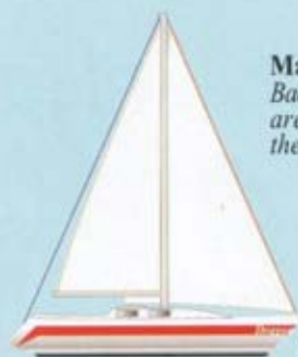
Fractional rig The forestay is attached some distance below the masthead.
